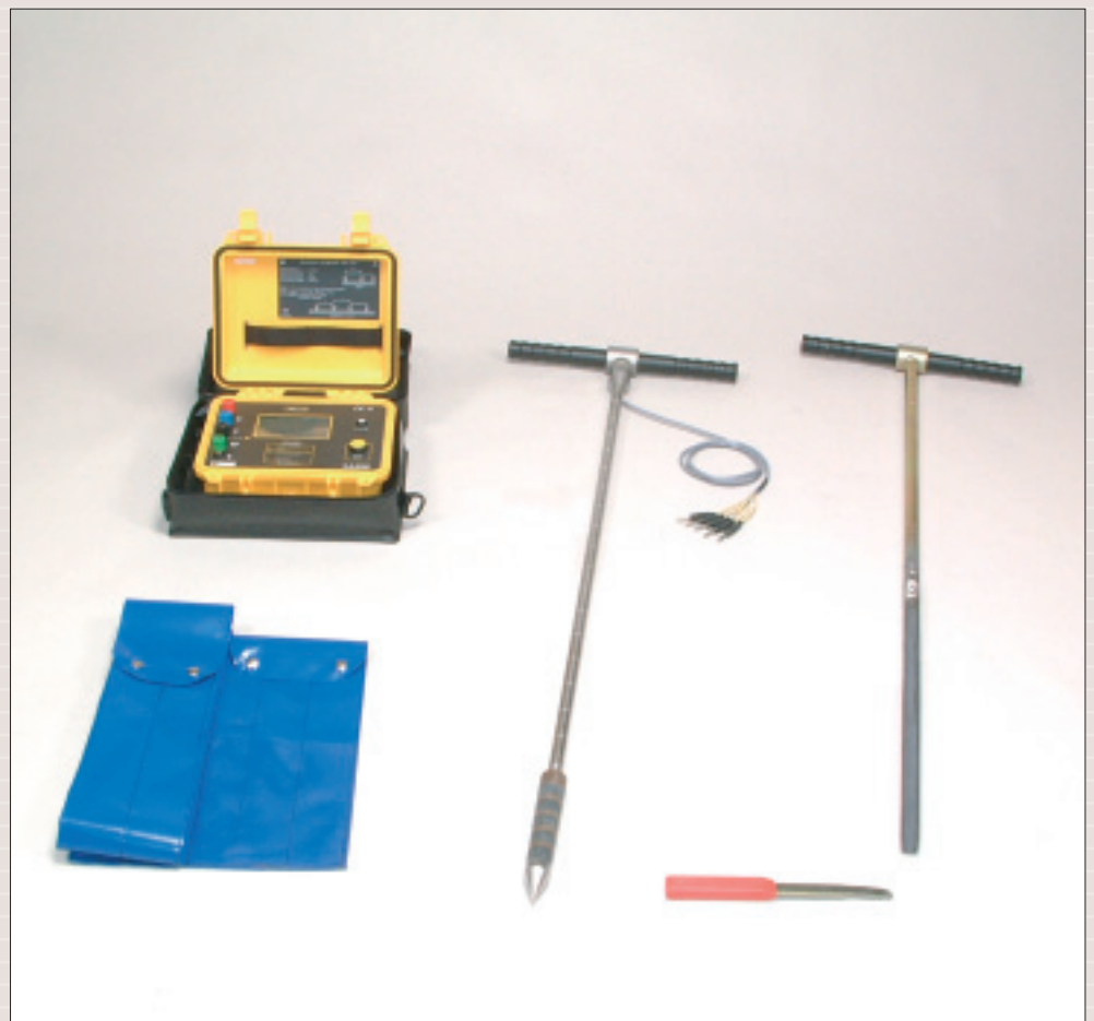
EC-probe for soil salinity measurements, standard set
